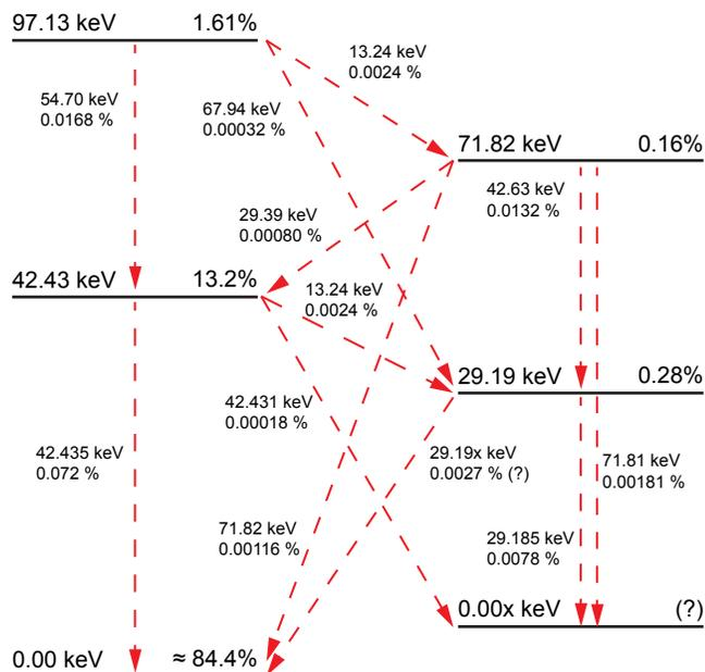
Figure 1: The first two bands in Th-229, showing their energies, and the population probability in U-233 alpha decay. Dashed lines represent gamma decay pathways.
